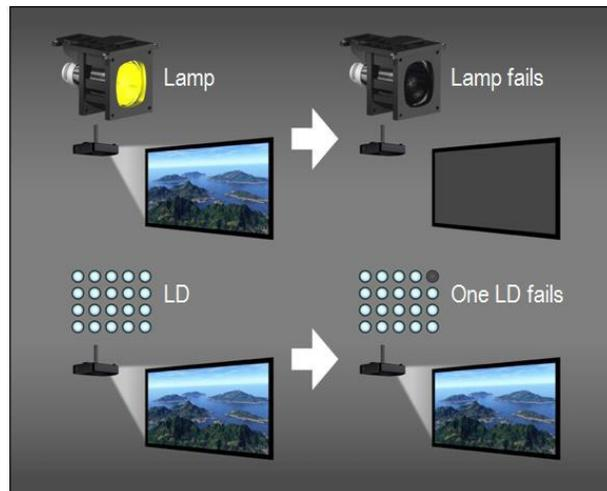
**Figure 4: A UHP Lamp Failure Causes a Dark Screen but a Laser Diode Failure only Reduces Brightness Slightly**
