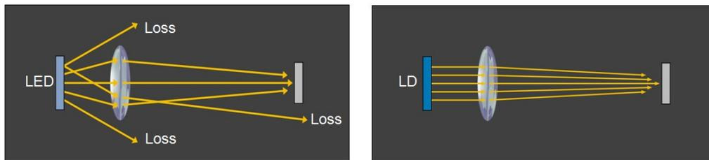
Figure 6: Collection of Light from an LED vs. a Laser Diode
