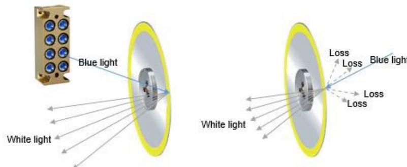
Figure 2: Reflective vs. Transmissive Laser Phosphor Wheel Designs
