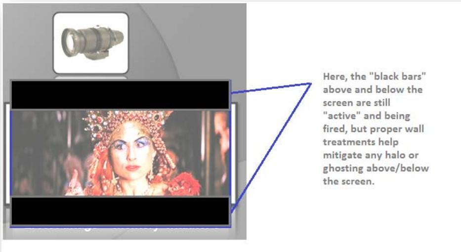
**3/ E-VariScope™, or Electronic VariScope.** We position the projector at its native optical throw distance so that you are filling the maximum width of the 2.35:1 screen. Somewhat similar to our zoom/lens memory method above (#2), we begin with the 16/9 black bars "overshooting" the top and bottom of the screen. The inner 2.35 content remains visible on screen.
