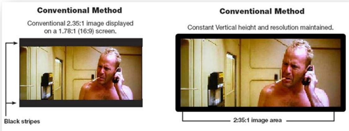
**2/ VariScope™ “lens memories” or lens indexing.** Here, the image is simply “zoomed out” so that the 2.35:1 content properly fills the full screen width; correspondingly the image is “zoomed in or down” to reduce the taller 16/9 content, in order to best fit the constant height screen. Pixels get slightly larger when watching ‘Scope content, slightly smaller when returning to 16/9.
